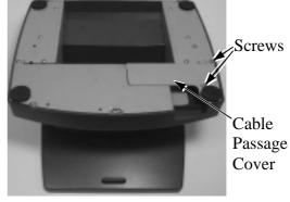
Now, unscrew the 2 screws on the cable passage cover and take the cable passage cover away to show the cable passage.
